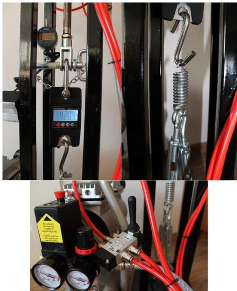
Fig. 2 The test stand – the spring with measurement devices: the crane scale and the dial indicator
